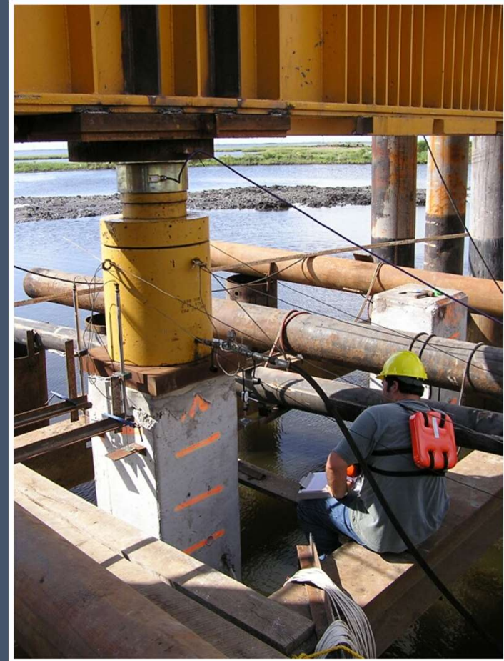
Reading Dial Gauges During Static Test
